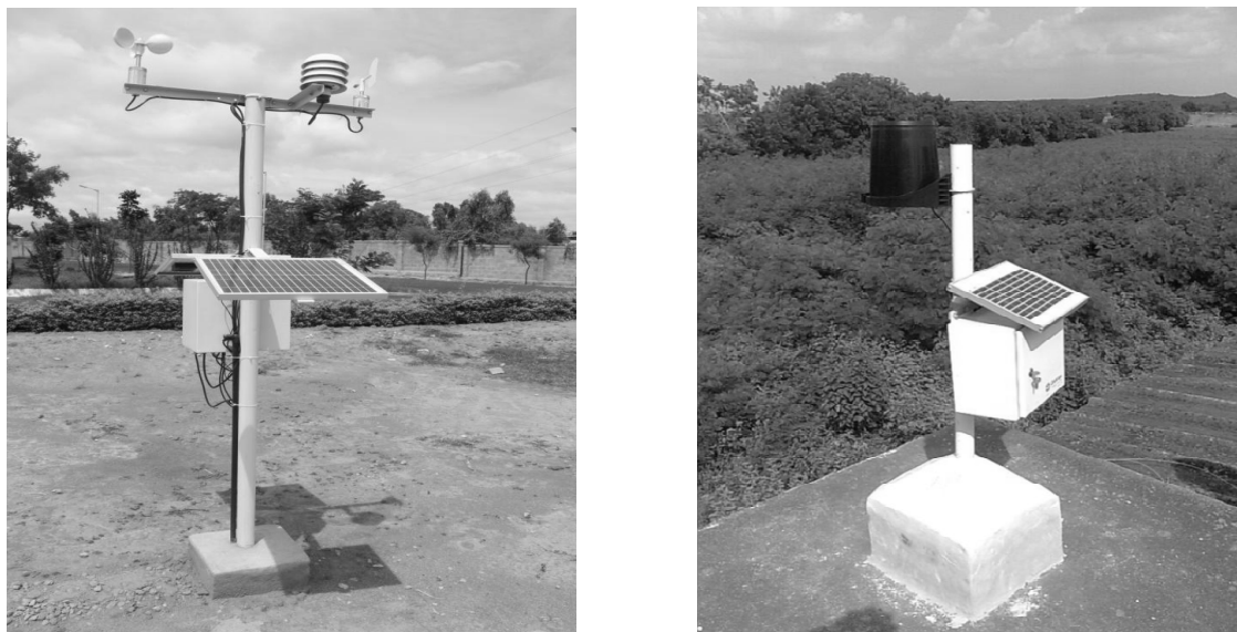
Fig 5. The pictures of (a) Solar Powered & GPRS enabled Telemetric Weather Station (TWS) and (b) Telemetric Rain Gauge Station (TRG) installed by KSNDMC in the state.
