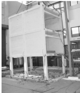
Fig. 1 Shake table test of OGS model frame
